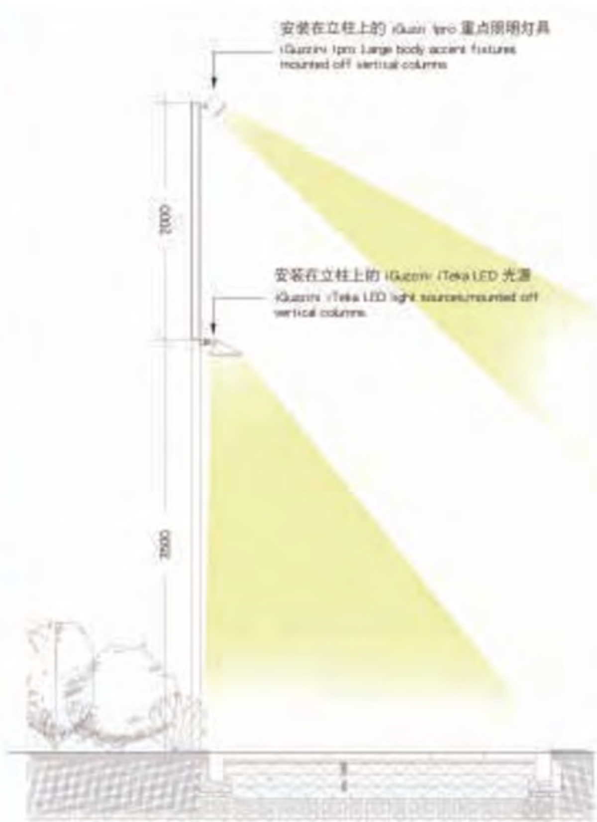
图 9b: 路灯照明设计图 Picture 9b: The light sketch of the roadway
